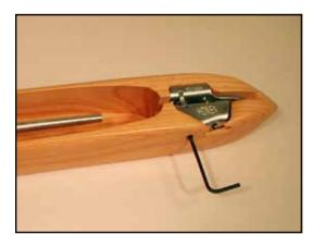
The Honex tensioner is quickly adjusted to properly tension yarn in a wide range of sizes.
